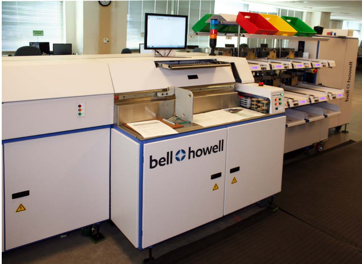
Front view showing work station where unopened ballots are placed and PC terminal. Colored trays indicate “good” ballots (in green trays that are ready to be furthered processed), “yellow” trays that indicate a sorting problem, and “red” trays where ballots are rejected and need further processing.
