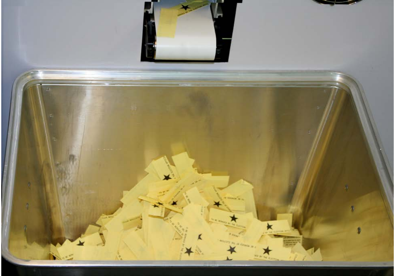
Security tabs that have been meticulously removed by a cutting laser operation are collected in this waste bin. Heat and fumes that are a by-product of this operation are vented outside the building.
